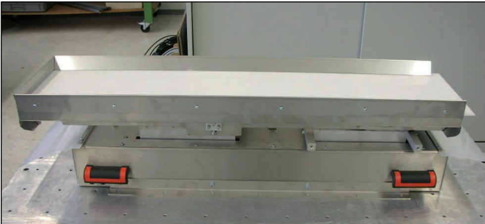
Figure 6-11: Mounting V-rails and Side Panels
